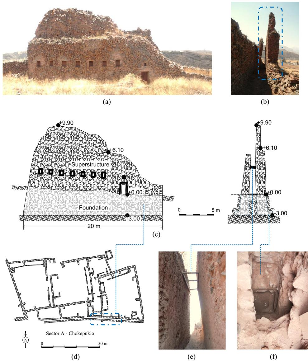
**Fig. 2.** General views of the studied area: (a) façade of the instrumented wall, (b) elevation of the instrumented wall, (c) front and transversal sections of the studied structure, (d) plan of the studied sector adapted from [12], (e) internal view of the two studied walls and (f) foundation detail.
